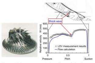
Fig. 4 High pressure ratio impeller and shock wave measurement
