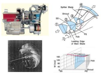
Fig. 1 Passenger car turbocharger, and LDV measurement for a large scale model of an actual impeller
