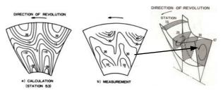
Fig. 5 Radial turbine flow measurement
