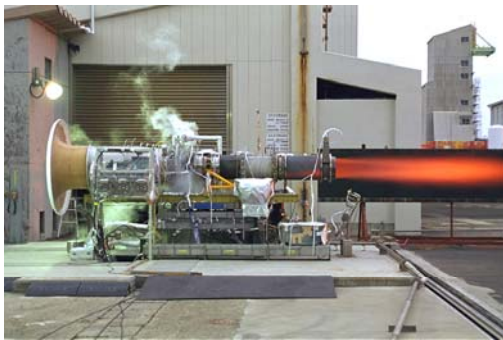
Fig. 3 Firing test of ATREX-500 engine
