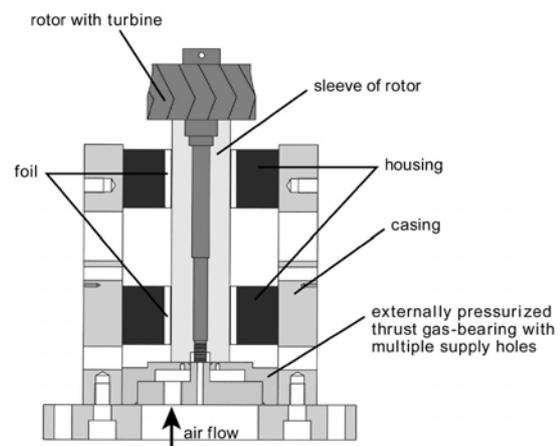
Fig.2 Radial Foil Bearing Test Setup
