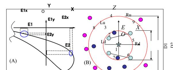
**Fig. 1 Interface construction method. (A) Selection of interpolation plane, (B) detection of CFD nodes, ☆ : FEM node E, ○ : CFD node.**
