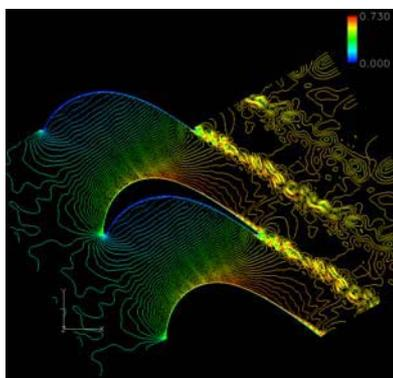
**Fig. 4 Contour of Mach number around the turbine blade**
