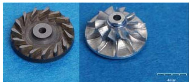
**Fig. 5 Prototype of radial turbines ( $\phi$  8 mm)**
