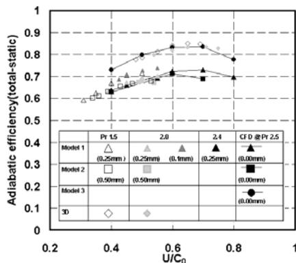
**Fig. 3 Measured total-to-static adiabatic efficiency of test turbines**
