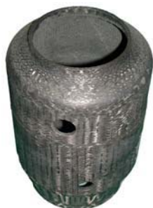
Fig. 1 CMC Combustor Liner
