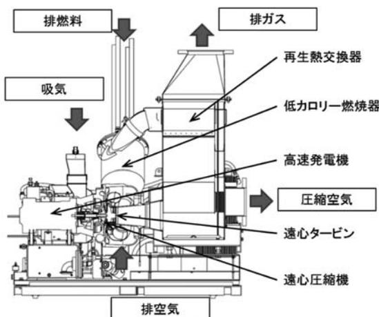
Fig. 4 Micro Gas Turbine cross section view
