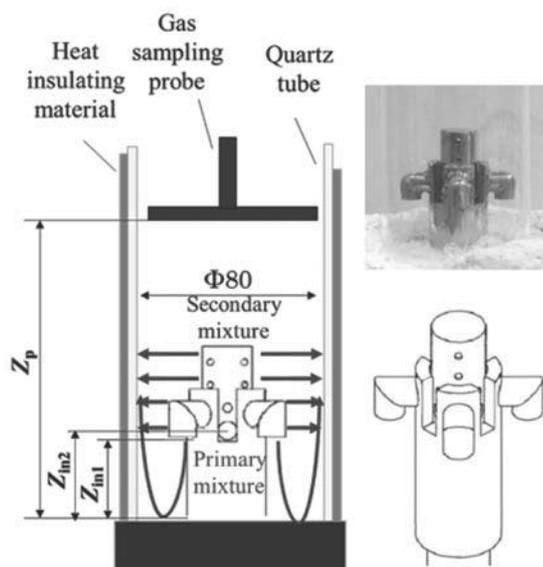
Fig. 1 Photographs and drawings of injectors used.
