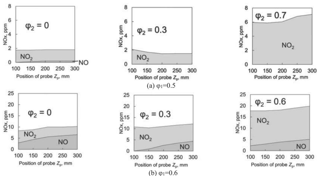
Fig. 10 Concentration of NO and NO<sub>2</sub> along the combustor axis for secondary mixture of different primary equivalence ratios for  $\phi_1$  of 0.5 and 0.6.
