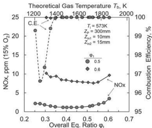
Fig. 8 NOx emissions corrected to 15% O<sub>2</sub> and combustion efficiency vs. overall equivalence ratios,  $\phi_o$ , for primary equivalence ratios,  $\phi_1$ , of 0.5 and 0.6.
