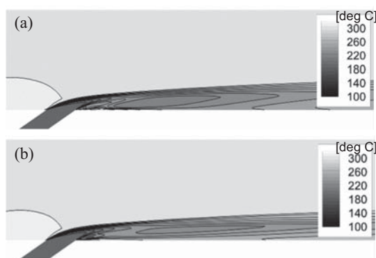
Fig. 8 Temperature distribution on a central slice, (a) SST original, (b) SST estimated
