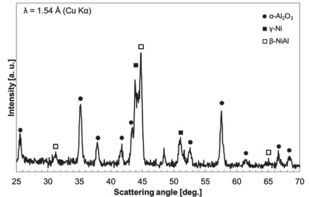
Fig. 3 XRD pattern of NiCoCrAlY surface after pre-oxidation at 1080 °C for 4 hour in vacuum (before in-situ XRD oxidation measurements)
