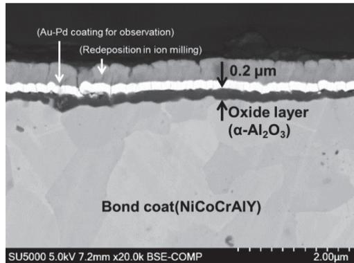
Fig. 2 Cross-section SEM image of NiCoCrAlY surface after pre-oxidation at 1080°C for 4 hour in vacuum (before in-situ XRD oxidation measurements)
