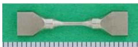
Fig.1 Specimen shape of low-cycle fatigue tests (mm)
