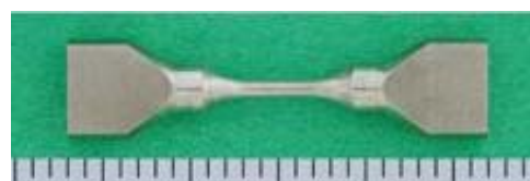
Fig.1 Specimen shape of low-cycle fatigue tests (mm)
