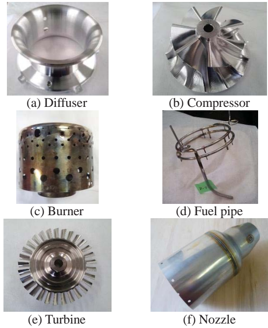
Fig. 3 Components of the NSP engine
