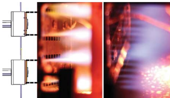
Fig. 9 Atmospheric micro-mix burner hydrogen combustion test hydrogen flame with 1.0mm injection holes
