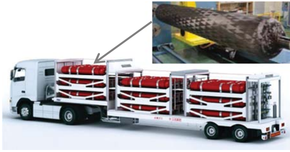
Fig. 5 Hydrogen gas carrier with 45MPa gas bottles
