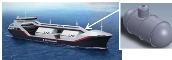
Fig. 4 Image of liquid hydrogen carrier and tank
