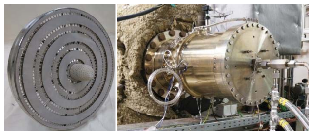
Fig. 9 Prototype of Micro-Mix burner module and combustor installed into IKDG test facility
