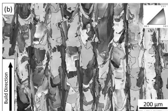
Fig. 4 IPF maps (Z direction) of as-built specimens on X plane of (a)67/67 block and (b)90/90 block.
