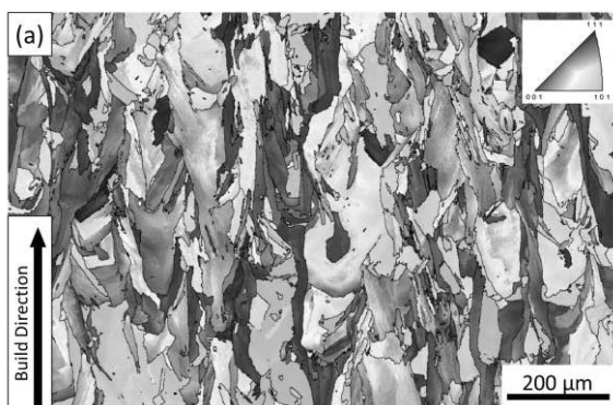
Fig. 3 IPF maps (Z direction) of as-built specimens on Z plane of (a)67/67 block and (b)90/90 block.
