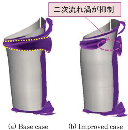
Fig.13 Visualization of Q-constant plane (purple color) near the 2nd stage stator from CFD
