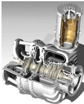
Fig. 3 Schematic view of Kawasaki M1A-17 gas turbine
