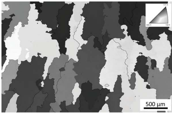
Fig. 5 IPF map of the cast specimen.
