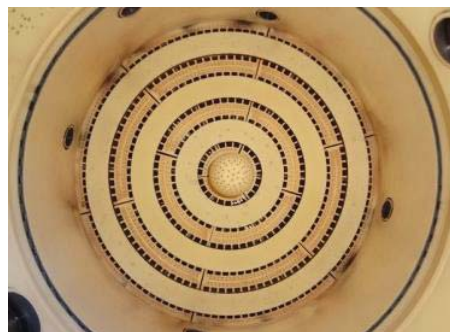
Fig. 12 Image of inside the combustor after high pressure combustion tests
