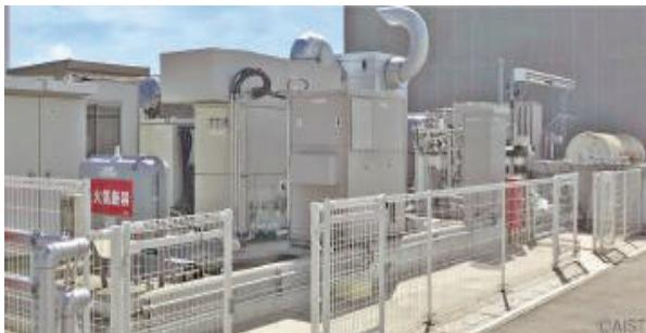
Fig.1 Ammonia Combustion Gas Turbine Test Rig
