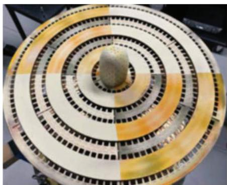
Fig. 12 Micro-mix burner module after engine demonstration tests
