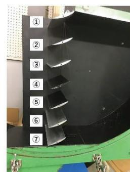
Fig. 1 Test section of linear cascade wind tunnel
