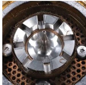
Fig. 2 Picture of a swirler ( $Sg=0$ ) and an injector
