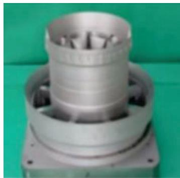
Fig. 11 Prototype of swirl block for gas turbine combustor produced by Additive manufacturing technology<sup>(5)</sup>
