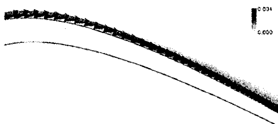
Fig. 7 Turbulence kinetic energy distribution near the suction surface (turbulence intensity 5%)
