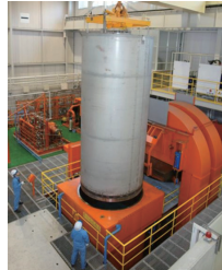
The world's largest HIP unit. (Giga-HIP)
