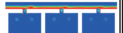
Fig. 2 Instantaneous vorticity contours of acoustic liner (3 resonators) under grazing flow by aeroacoustic simulation
