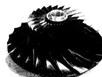
Fig. 6 Strong backscatter test impeller ( N_s = 24 )
