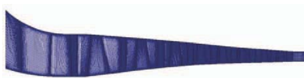
Fig. 3 CFD analysis full stage mesh
