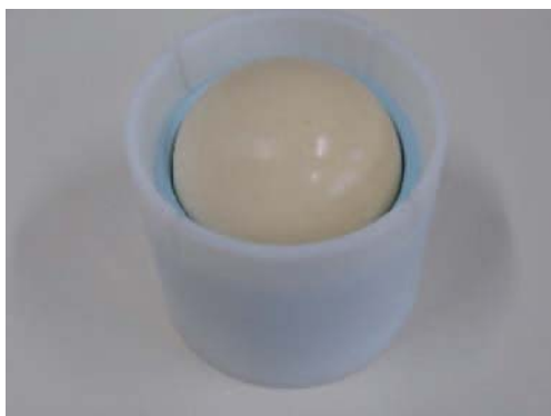
Fig. 6 The gelatin ball held in sabot
