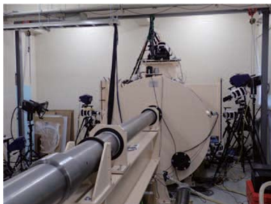
Fig. 8 Arrangement of high-speed video cameras and lighting equipment
