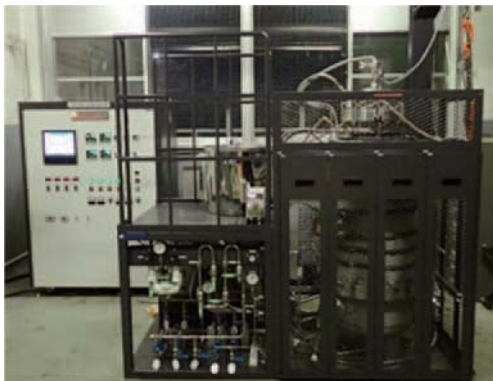
Fig. 11 Durability test apparatus in high temperature water vapor environment
