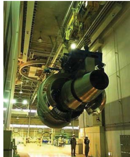
Fig. 6 Engine conveyed by crane
