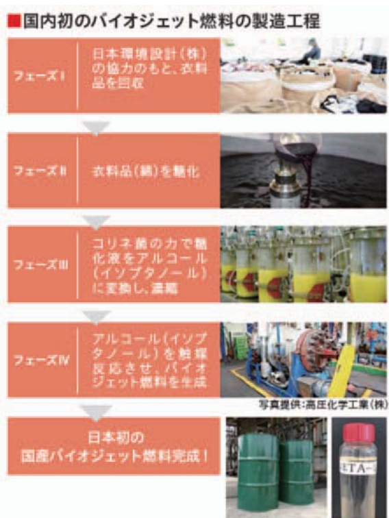
Fig. 3 Process to Produce SAF made from Cotton Clothes
