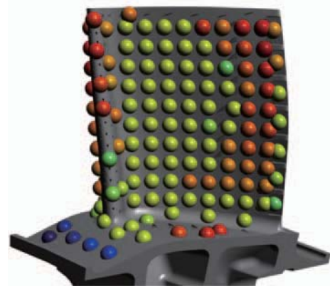
Fig. 10 Temperature distribution obtained with THC
