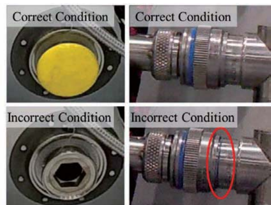
Fig. 6 Parts assembled and their defective portions
