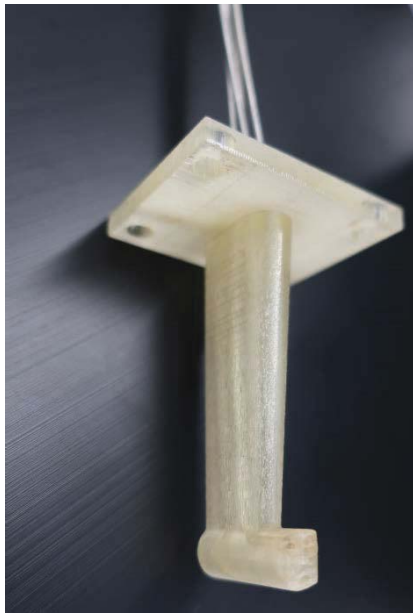
Fig. 1 Additive manufacturing multi hole probe with temperature measurement
