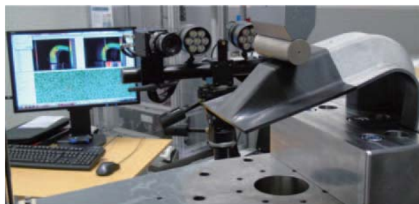
Fig. 17 Test setup for fiber-reinforced PA6 plastic parts
