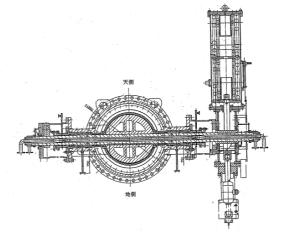
Fig. 5 Cross section of gas shut-off valve
