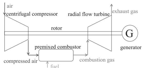
Fig. 1 System diagram of objective turbine
