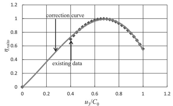
Fig. 5 Correction curve of radial flow turbine efficiency
