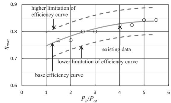
Fig. 4 Maximum efficiency curves of radial flow turbine
