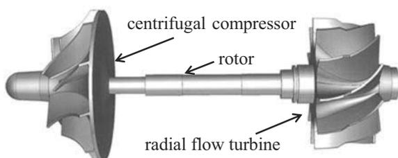
Fig. 7 Side view of the turbine rotor
