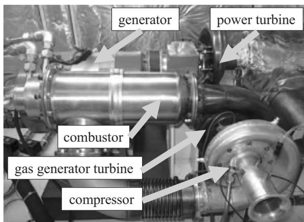
Fig. 6 Outside of reference microturbine for verification
