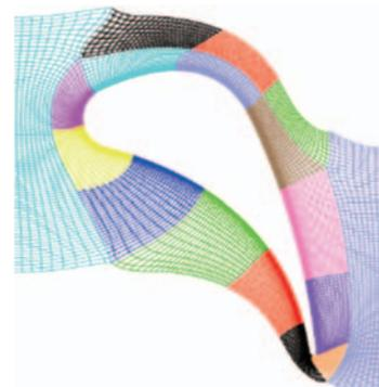
Fig. 3 Grid around Original vane
